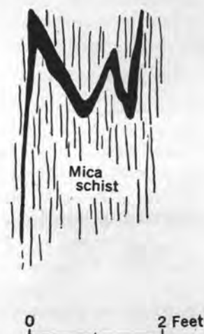
FIGURE 35.—Detailed sketch of quartz veinlet crosscutting foliation planes of the mica schist, Kin Mori mine, Dawson County, Ga.
