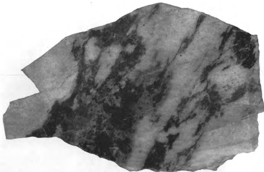
B. BANDED ORE FROM LOCKHART MINE, GEORGIA. White, quartz; gray, amphibole; black, garnet and chlorite. Polished slab.
