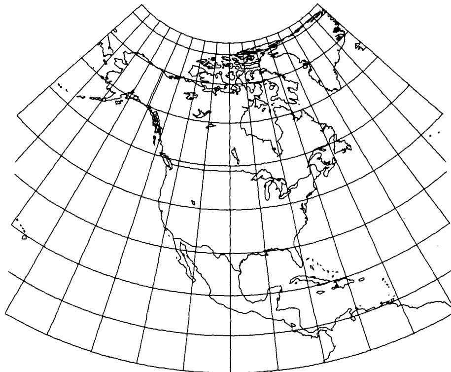
FIGURE 20.—Albers Equal-Area Conic projection, with standard parallels 20^{\circ} and 60^{\circ} N. This illustration includes all of North America to show the change in spacing of the parallels. When used for maps of the 48 conterminous States standard parallels are 29.5^{\circ} and 45.5^{\circ} N.
