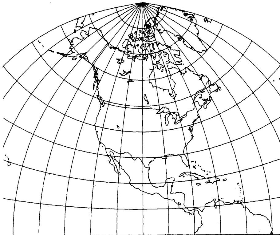
FIGURE 25.—North America on a Polyconic projection grid, central meridian long. 100^{\circ} W., using a 10^{\circ} interval. The parallels are arcs of circles which are not concentric, but have radii equal to the radius of curvature of the parallel at the Earth's surface. The meridians are complex curves formed by connecting points marked off along the parallels at their true distances. Used by the USGS for topographic quadrangle maps.
