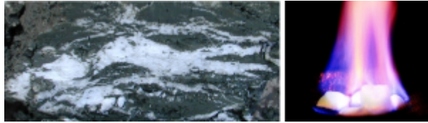
Figure 18.11 Left: Methane hydrate within muddy sea-floor sediment from an area offshore from Oregon. [ https://upload.wikimedia.org/wikipedia/commons/4/49/Gashydrat_im_Sediment.JPG ] Right: Methane hydrate on fire [ http://www.usgs.gov/blogs/features/files/2012/01/New-Image.jpg ]
