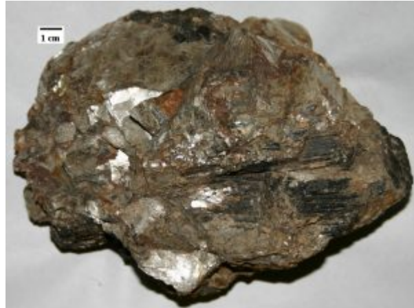
Figure 3.18 A pegmatite with mica, quartz, and tourmaline (black) from the White Elephant mine, South Dakota [from http://en.wikipedia.org/wiki/Pegmatite#mediaviewer/File:We-pegmatite.jpg ]
