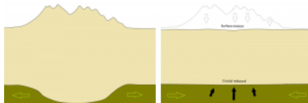
Figure 9.17 Illustration of the isostatic relationship between the crust and the mantle. Following a period of mountain building, mass has been added to a part of the crust, and the thickened crust has pushed down into the mantle (left). Over the following tens of millions of years, the mountain chain is eroded and the crust rebounds (right). The green arrows represent slow mantle flow. [SE]
