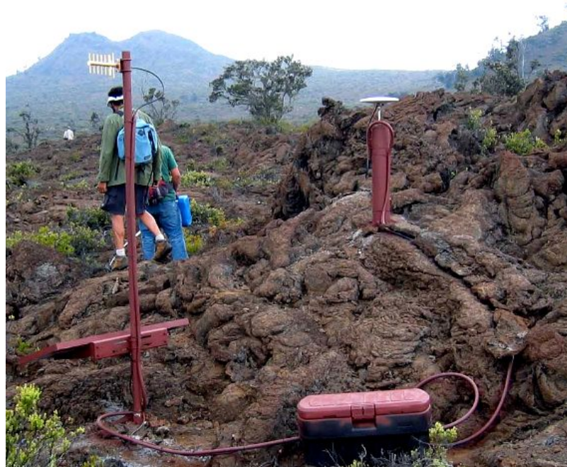
Figure 4.27 A GPS unit installed at Hualalai volcano, Hawaii. The dish-shaped antenna on the right is the GPS receiver. The antenna on the left is for communication with a base station. [from USGS at: http://hvo.wr.usgs.gov/volcanowatch/view.php?id=173 ]
