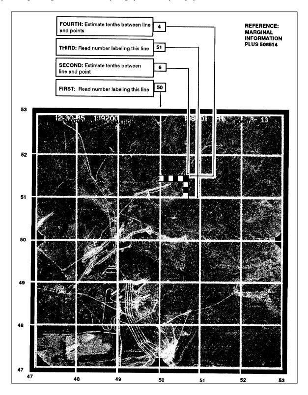
Figure 8-18. Reading point designation grid coordinates
