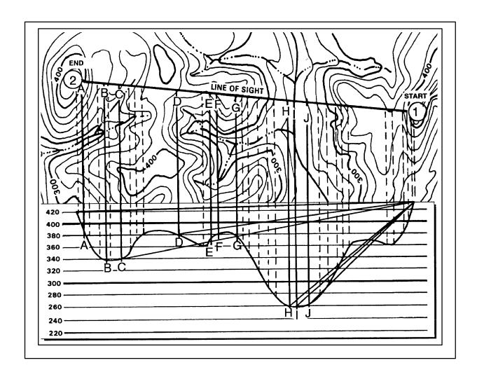
Figure 10-30. Drawing lines to additional points.
