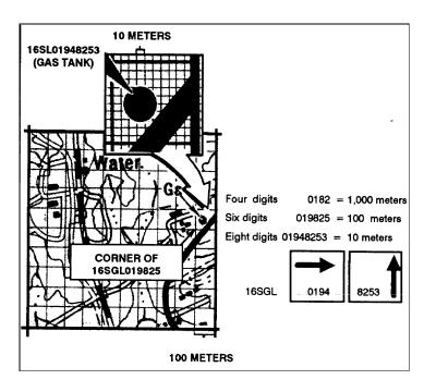
Figure 4-18-C. The 100-meter and 10-meter grid squares.
