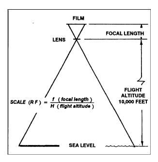
Figure 8-10. Basic computation of scale from sea level.
