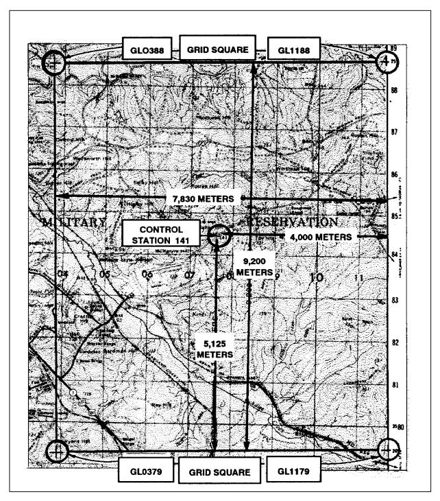
Figure 4-7. Using the proportional parts method.
