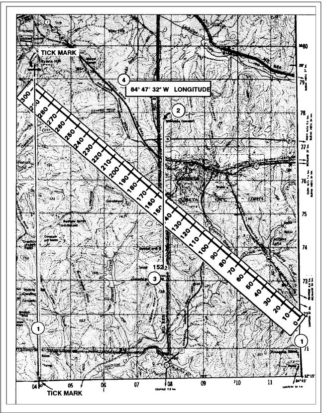
Figure 4-5. Determining longitude.
