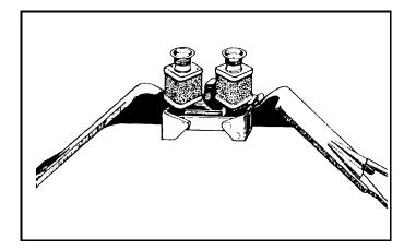
Figure 8-23. Mirror stereoscope.
