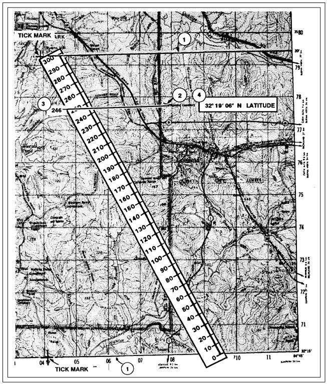
Figure 4-4. Determining latitude.
