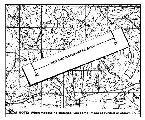
tenths (Figure 5-4). As you break down the distance between the squares in the extension scale into tenths, you will see that tick mark (a) is aligned with the 950-meter mark. Adding the distance of 3,000 meters determined in the primary scale to the 950 meters you determined by using the extension scale, we find that the total distance between points (a) and (b) is 3,950 meters.
