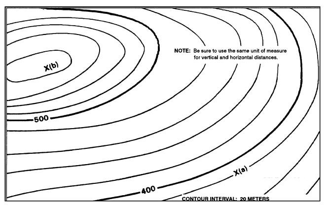
Figure 10-11. Contour line around slope.
