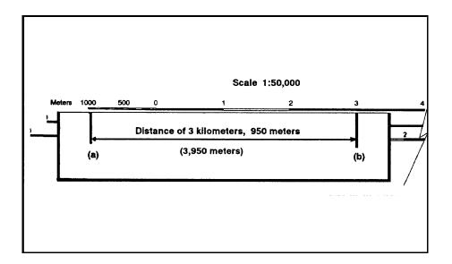
Figure 5-4. Measuring straight-line map distance.
