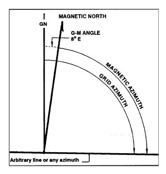
Figure 6-9. Declination diagram with arbitrary line
