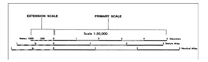
Figure 5-2. Using a graphic (bar) scale.
