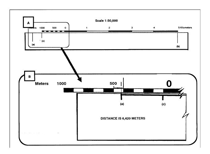
Figure 5-6. Determining the exact distance.
