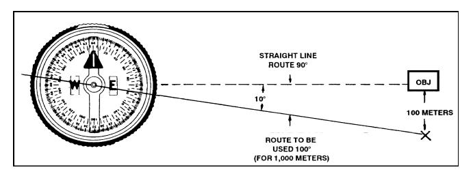
Figure 9-6. Deliberate offset to the objective.
