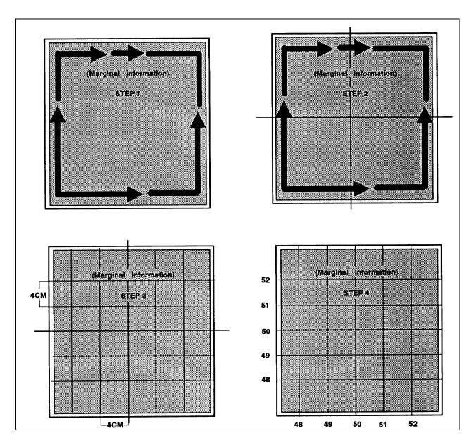
Figure 8-17. Constructing a point designation grid.
