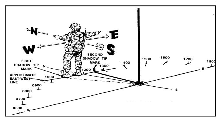
Figure 9-7. Determining directions and time by shadow.
