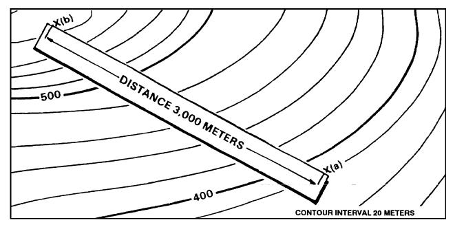
Figure 10-12. Measuring horizontal distance
