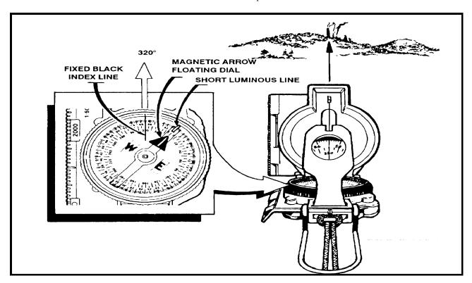
Figure 9-4. Compass preset at 320 degrees.
