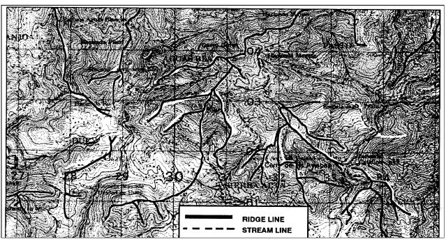
Figure 10-27. Ridgelining and streamlining.
