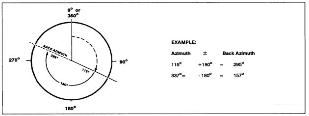
Figure 6-3. Back azimuth.
