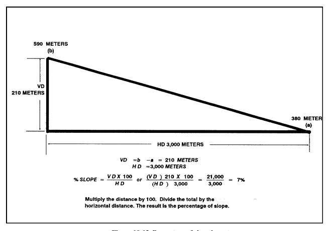
Figure 10-13. Percentage of slope in meters.
