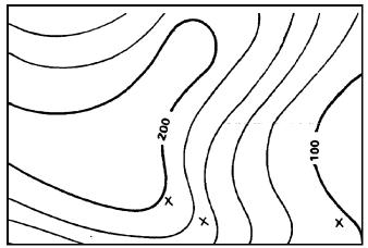
Figure 10-4. Points between contour lines.
