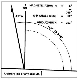
Figure 6-15. Converting to a grid azimuth when the G-M angle is greater.
