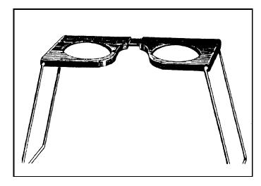
Figure 8-22. Pocket stereoscope.
