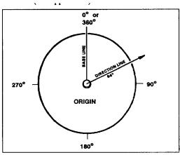
Figure 6-2. Origin of azimuth circle.
