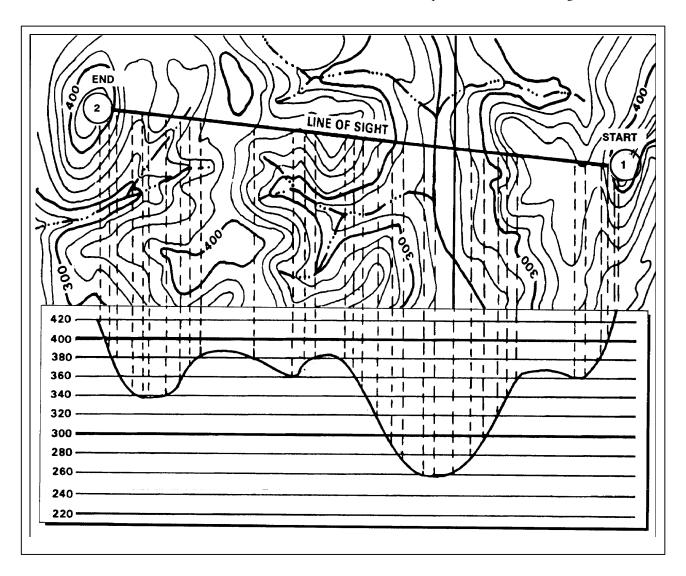
Figure 10-29. Dropping perpendiculars.
