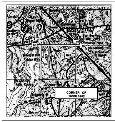
Figure 4-18B. The 1,000-meter grid square.
