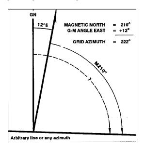
Figure 6-10. Converting to grid azimuth.
