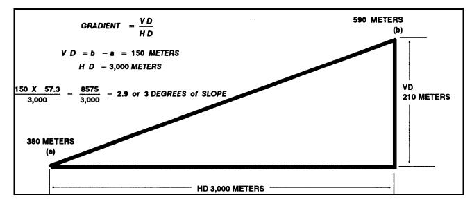
Figure 10-14. Degree of slope.
