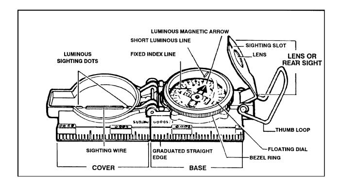
Figure 9-1. Lensatic compass.
