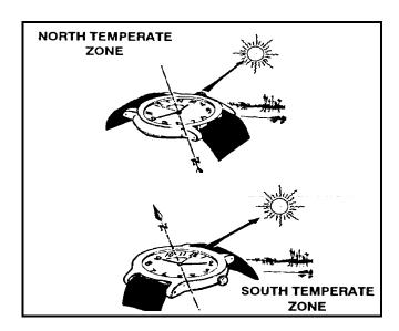
Figure 9-8. Determining direction by using a watch.
