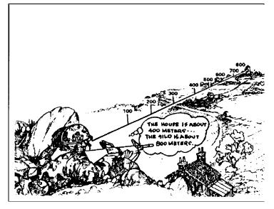
Figure 5-9. Using a 100-meter unit-of-measure method.
