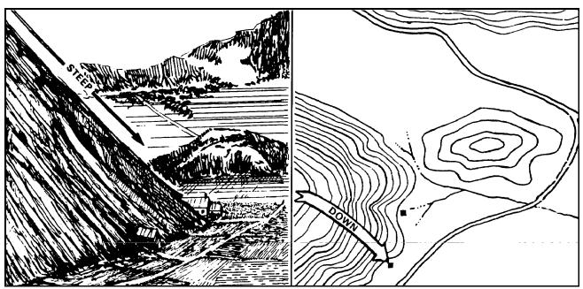
Figure 10-7. Uniform, steep slope.
