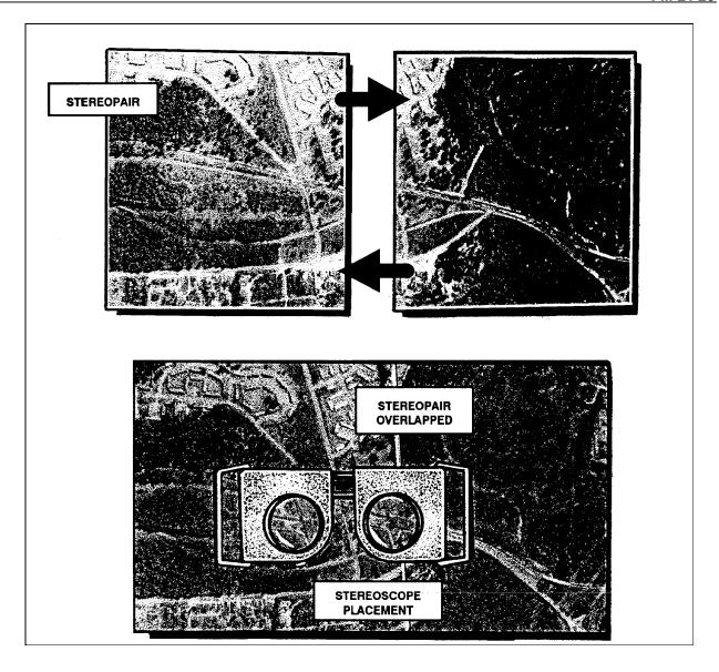
Figure 8-24. Placement of stereoscope overstereopair.
