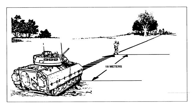
Figure 12-4. Determining an azimuth, dismounted.
