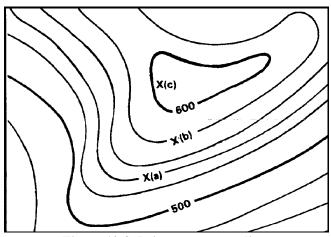
Figure 10-3. Points on contour lines
