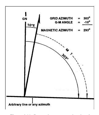
Figure 6-11. Converting to magnetic azimuth.
