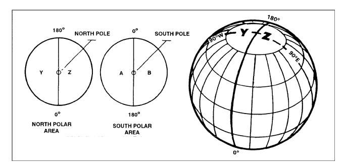
Figure 4-10. Grid zone designation for UPS grid.
