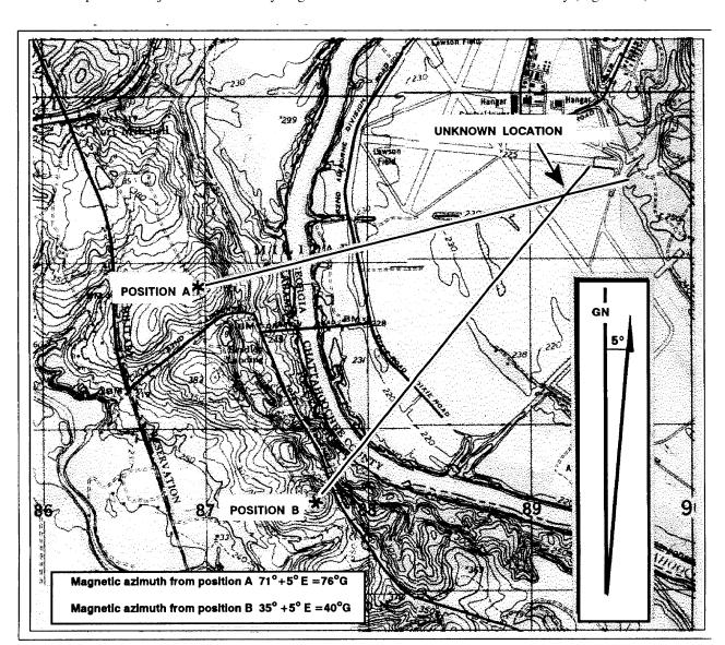
Figure 6-16. Intersection, using map and compass.
