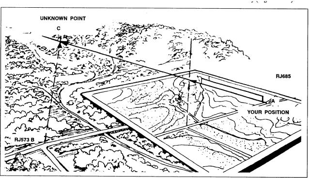
Figure 6-17. Intersection, using a straightedge.
