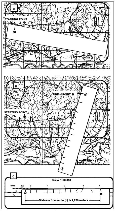
Figure 5-5. Measuring a curved line.
