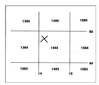
Figure 4-15. Determining grids without coordinate point.
