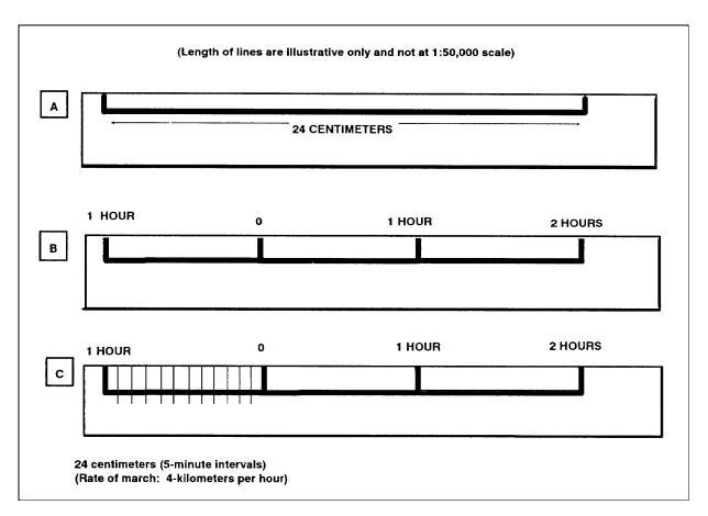
Figure 5-8. Constructing a time-distance scale.
