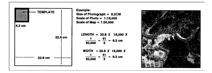
Figure 8-13. Constructing a template.
