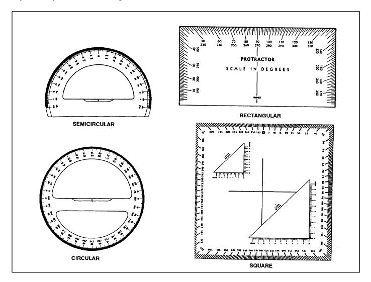
Figure 6-5. Types of protractors.
