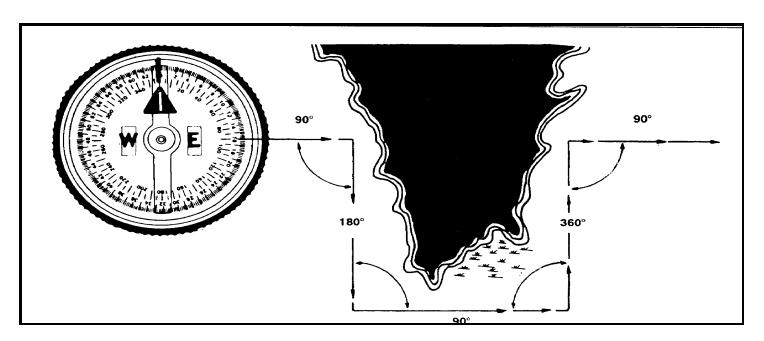
Figure 9-5. Bypassing an obstacle.
