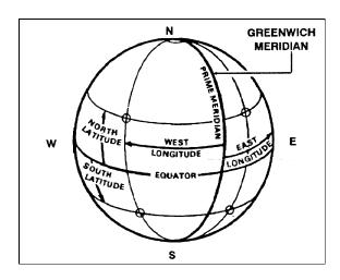
Figure 4-1. Prime meridian and equator.
