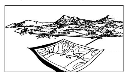
Figure 5-1. Converting map distance to ground distance.
