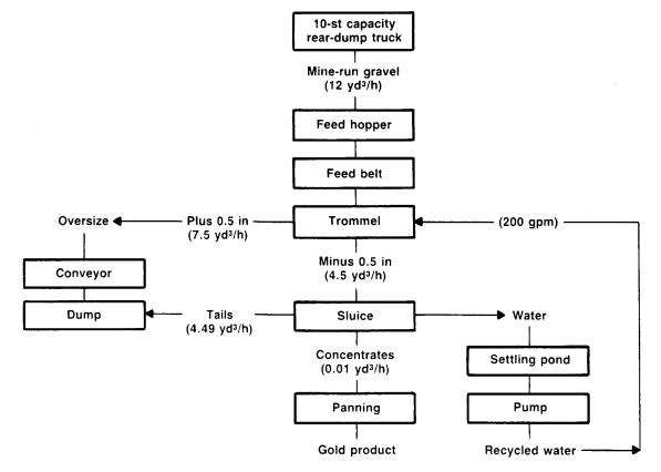
Figure 1.—Sample flow sheet, sluice mill.
