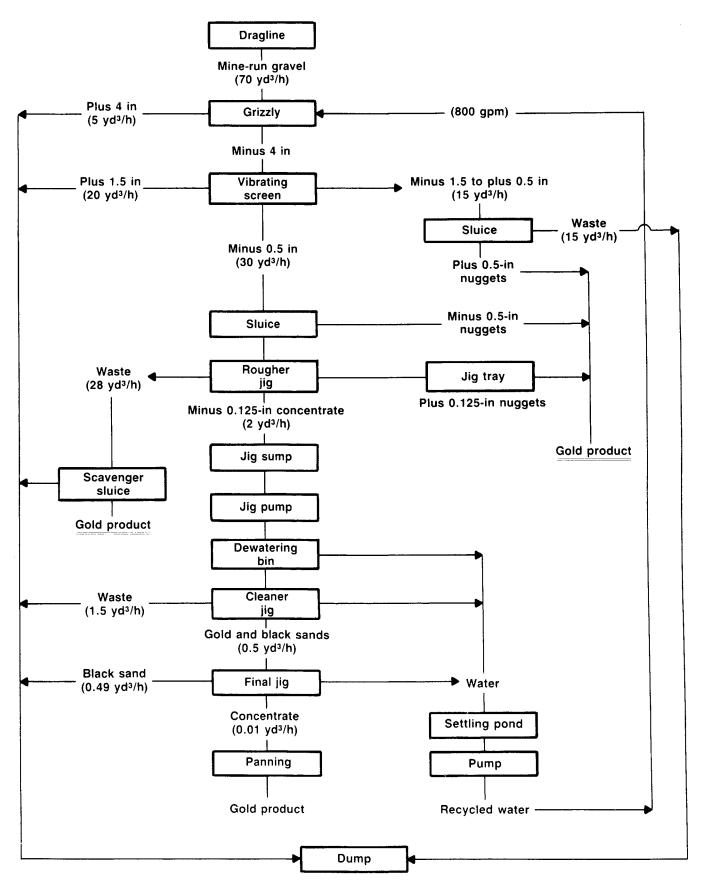
Figure 2.—Sample flow sheet, jig mill.
