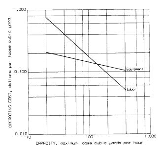
Processing operating costs - tailings removal - Front-end loaders
