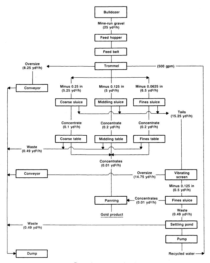
Figure 3.—Sample flow sheet, table mill.
