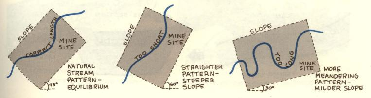
**Bed Stability:** The bed stability of a rehabilitated stream should approximate the stability of a natural stream with the same stream pattern. The type of stream determines the degree of bed stability needed. A meandering stream should have a stable bed up to 3/4 bankfull. A mountain stream should have a low sediment transport and a stable bed at bankfull conditions.
