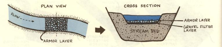
Bank Stability: Channel banks can be protected from erosion by revetment. Revetment will prevent lateral movement of the channel, but will also prevent plant regrowth, so use it only where necessary to stabilize the bank. Riprap of rubble or quarry stone is generally the most reliable and economical revetment.
