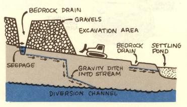
**Bedrock Drains:** Bedrock drains are used to collect groundwater that infiltrates the mine area. Two types of drains can be constructed: one that intercepts water above the mine area and diverts it into the stream or diversion channel, and one that collects water from within the work area and routes it to settling ponds.
